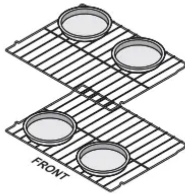
Figure 11: Pan positions two rack baking
