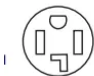
4-wire receptacle (14-30R)
