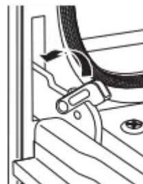
Push hinge locks down to lock
