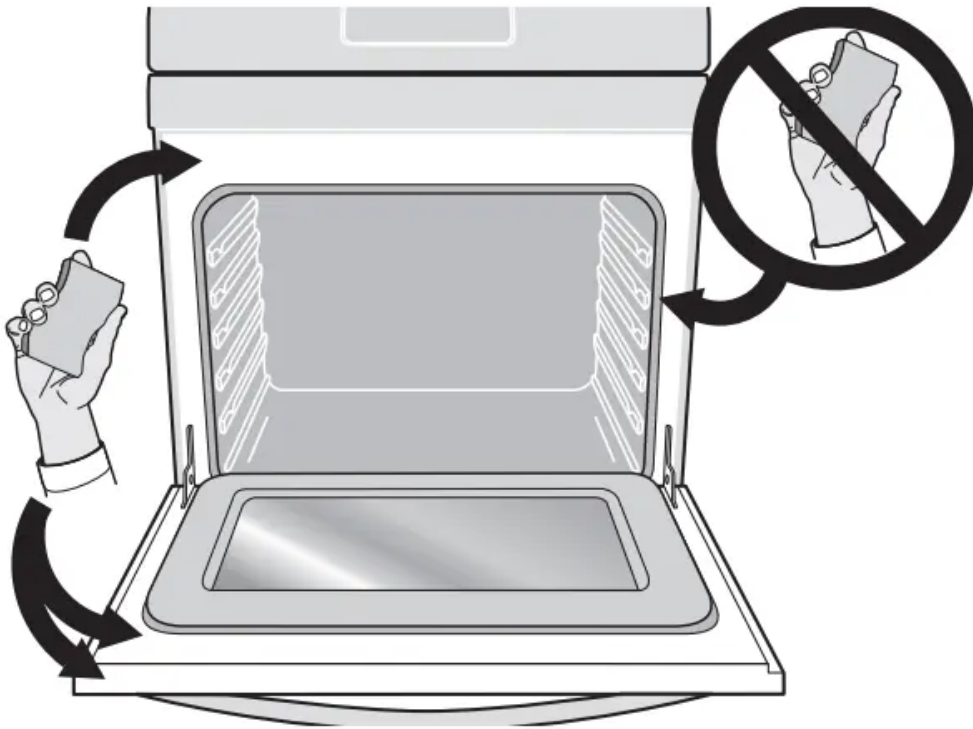
Figure 6: Clean around the oven door gasket
