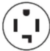
4-wire receptacle (14-30R)
