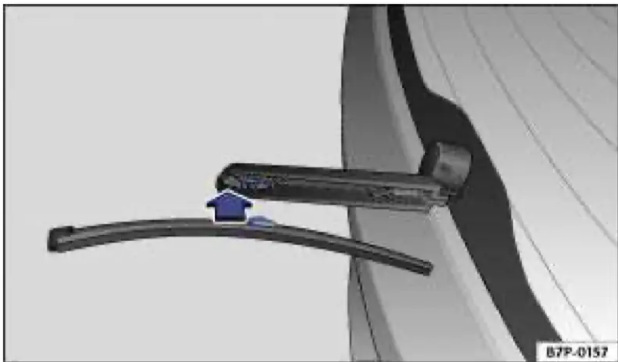
Fig. 322 Changing the rear window wiper blades.
