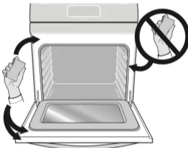
Figure 20: Clean around the oven door gasket
