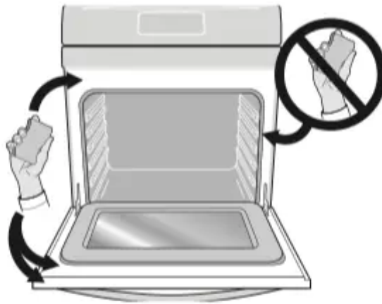
Figure 22: Clean around the oven door gasket
