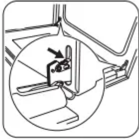
Figure 22: Door hinge location
