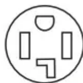
4-wire receptacle (14-30R)
