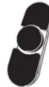
Dual Oval Burner (on some models) Use this burner to cook on the griddle or with small cookware.
