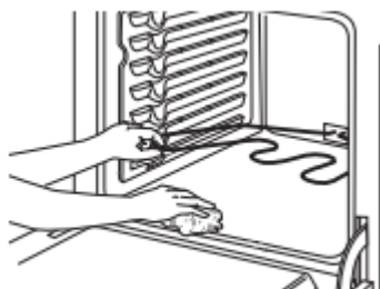
Gently lift the bake element
