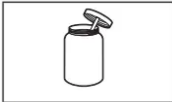
Pipe-joint compound resistant to propane gas
