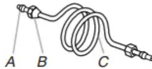
A. Compression sleeve C. Copper tubing B. Compression nut
