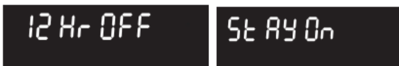
Figure 18: 12 hr energy saving (L) and continuous setting (R)
