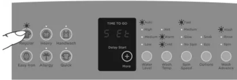
Fig.22 Customising a wash cycle, eg REGULAR cycle
