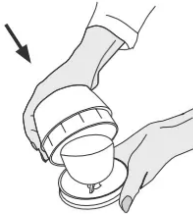
Fig.15 To separate, push cup away from dispenser with thumb
