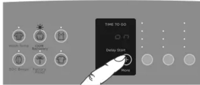
Fig.28 Changing the out of balance recovery routine
