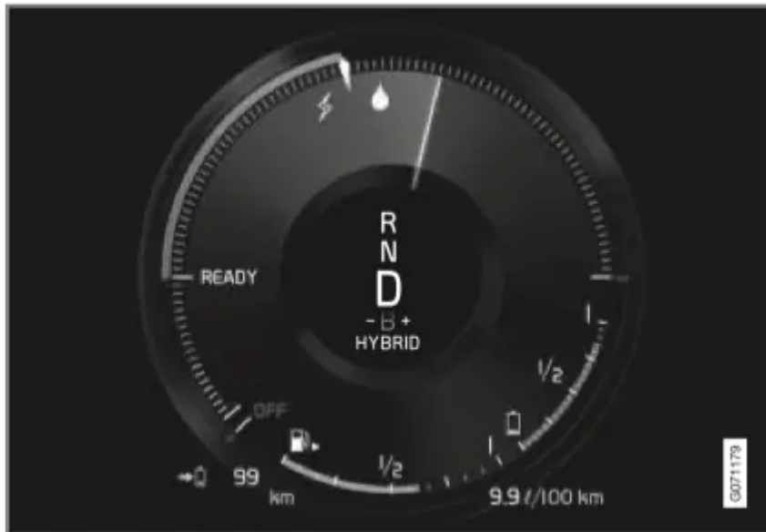
The driver display for propulsion with both the electric motor and internal combustion engine.
