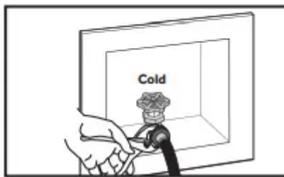
Cold Water Source Connection
