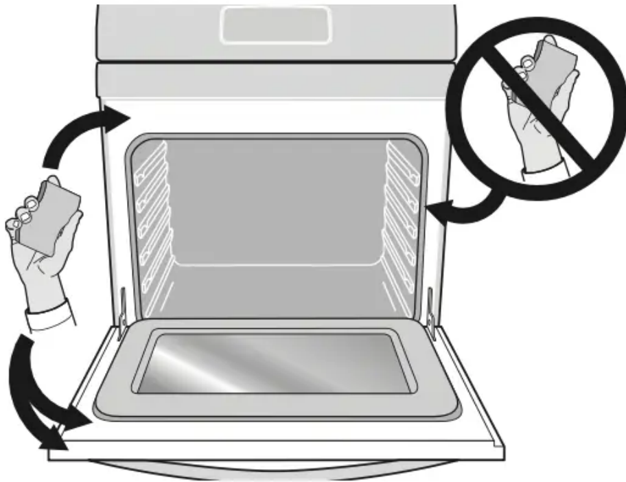
Figure 24: Clean around the oven door gasket
