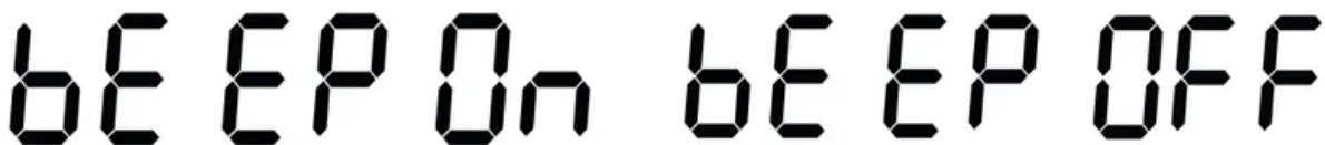
Figure 8: Display showing audible and silent operation
