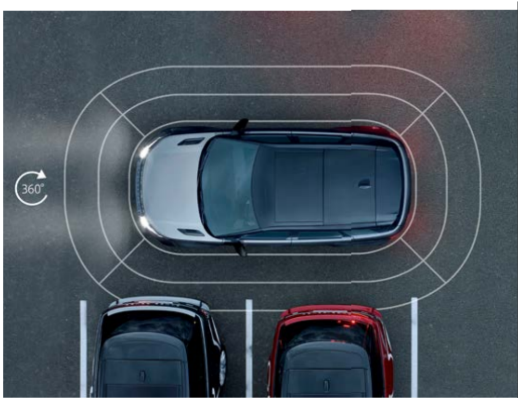
360° Surround Camera uses four digital cameras discretely placed around the vehicle, providing a 360° bird's-eye view on the Touchscreen. With the capacity to display several different views at
