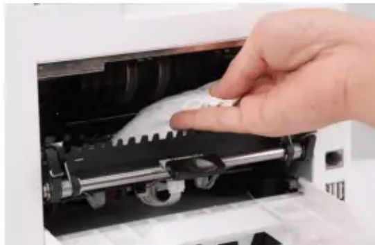
Figure 7-23 Clean the Upper CIS
