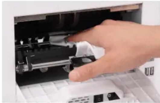
Figure 7-22 Clean the Lower CIS
