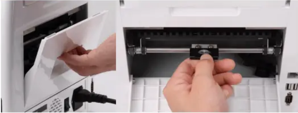
Figure 7-21 Open the Back Covers
