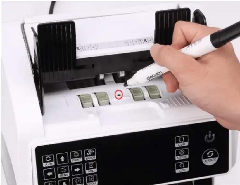
Figure 7-30 Use Marker Pen to Decrease the Sensitivity of Hopper Sensor
