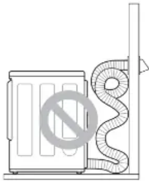
Excess or crushed transition duct
