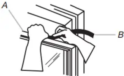
A. Top of lower window sash B. Foam seal
