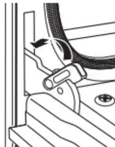
Push hinge locks down to lock
