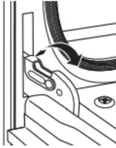
Pull hinge locks up to unlock
