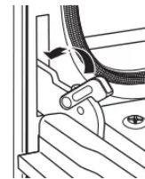
Push hinge locks down to lock
