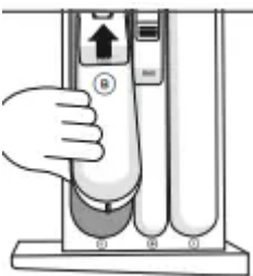
Replacing the liquid detergent compartment
