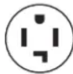
4-wire receptacle (14-30R)
