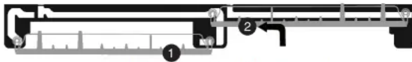
Left rack adjusted to lower position and right rack to upper position
