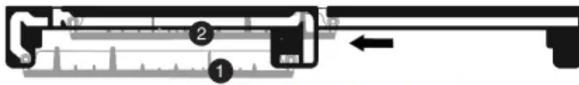
Left rack adjusted to lower position and right rack moved to the left
