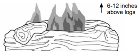
Fig. 30 - Incorrect/Abnormal Flame Pattern with tall flames
