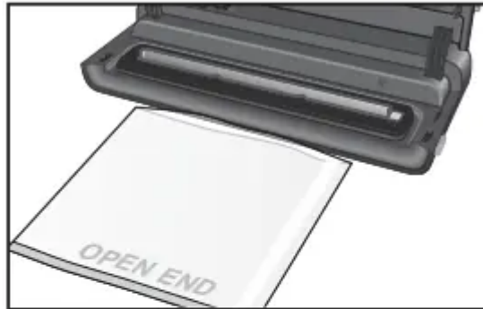
Place Bag on Sealing Strip
