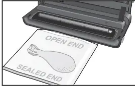
Place Bag in Vacuum Channel
