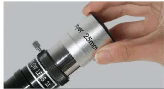
20. Insert 25mm eyepiece into 3X Barlow lens. (advise not use for viewing landscape)
