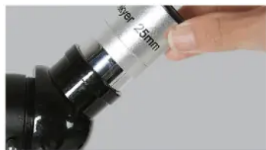
16. Insert 25mm eyepiece into zenith mirror.
