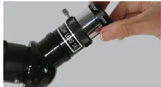
22. Insert 5mm eyepiece into 3X Barlow lens, (advise not use for viewing landscape)
