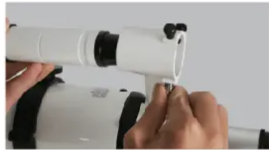
12. Pull down the metal stretching screw and slide finderscope into the hole on base.
