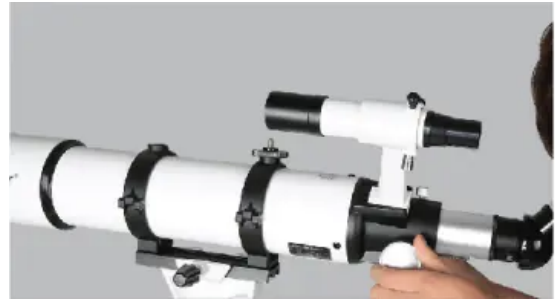
24. Turn the focuser wheel to make field clear.
