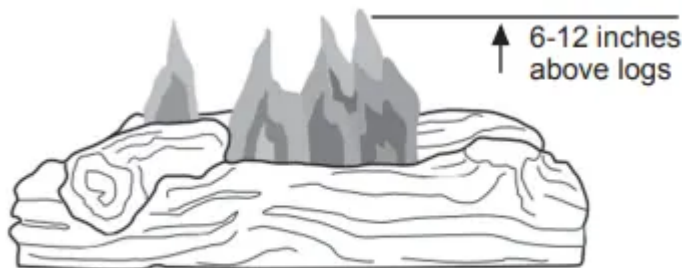
Fig. 32 - Incorrect/Abnormal Flame Pattern with tall flames
