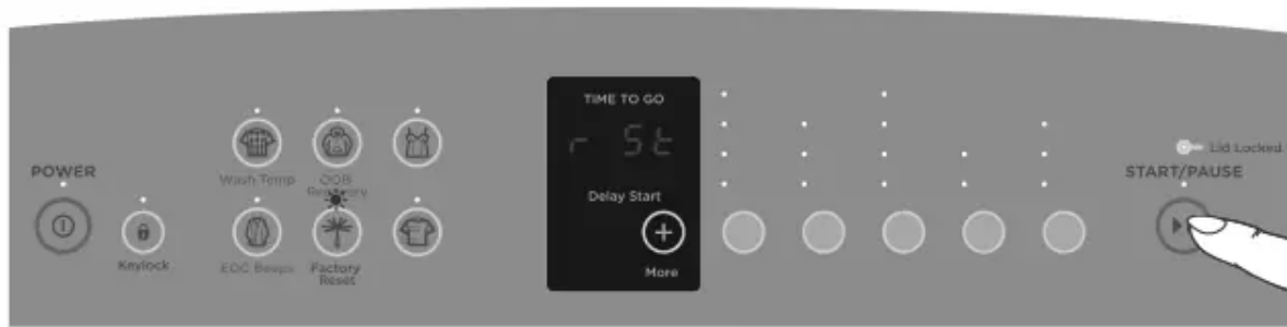
Fig.30 Changing the washer back to the factory default settings
