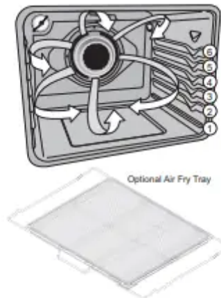
Figure 33: Optional Frigidaire Air Fry Tray. Use rack position 4 with tray or dark pan with low or no sides for best results.
