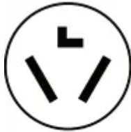
3-wire receptacle (10-30R)
