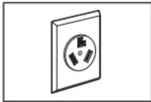
3-wire receptacle (NEMA type 10-30R)
