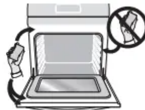
Figure 29: Clean around the oven door gasket
