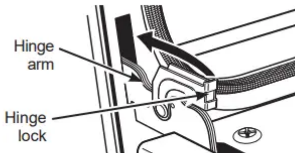
Push hinge locks up to lock
