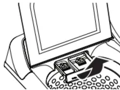
GTW680 and GTW685 models have a large dispenser drawer with compartments for both detergent and softener.
