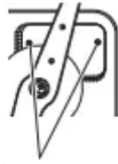
Sump cover screws
