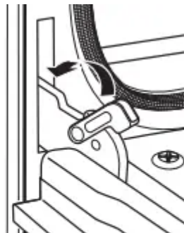
Push hinge locks down to lock
