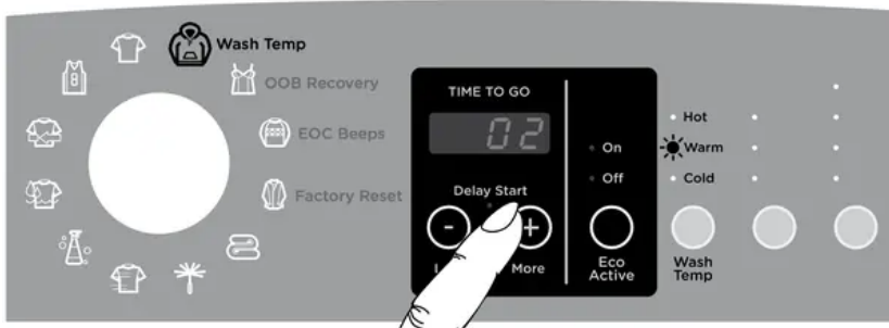
Adjusting the temperature setting, eg increasing the WARM wash temperature by 2°C
