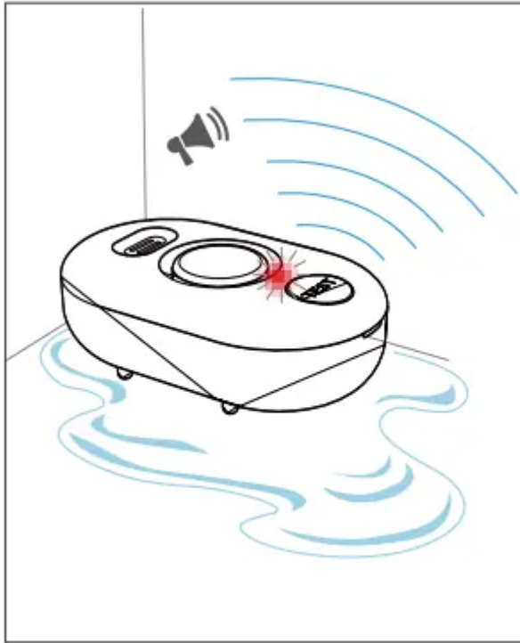
Water seepage Alarm
