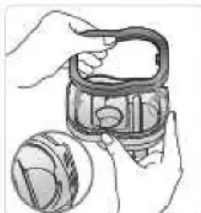
1. As shown in the picture, fit the rubber gasket into the groove and insert it.
