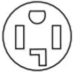
4-wire receptacle (14-30R)
