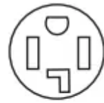
4-wire receptacle (14-30R)
