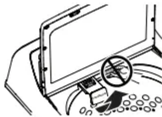
GTW840 and GTW845 models have a small dispenser drawer with one compartment for softener/conditioner only.
