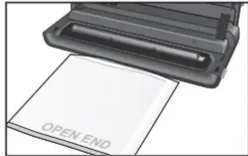
Place Bag on Sealing Strip
