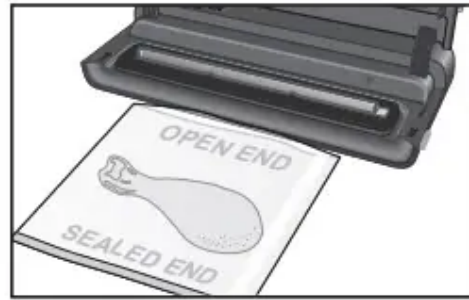
Place Bag in Vacuum Channel
