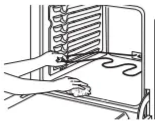
Gently lift the bake element
