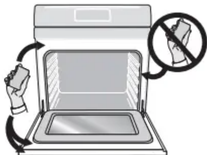
Figure 12: Clean around the oven door gasket
