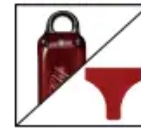
STEP 4. STORE STORE CLIPPER USING HANG HOOK IF PROVIDED AND COVER BLADES WITH RED BLADE GUARD DO NOT WRAP CORD AROUND CLIPPER
