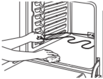
Gently lift the bake element
