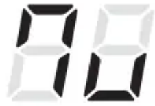
Duct Mode OFF
